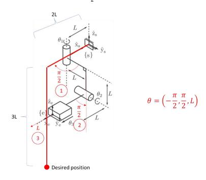
Alternatively, we can solve linear equations by formulating the FK equations and solve for the  $\theta$ . In this case we will determine the FK for the end-effector pose wrt {s},  $T_{se}(\theta)$  and equate it to the desired pose T.
