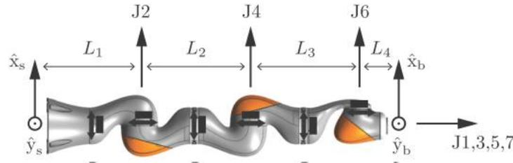
We can see that {b} at home configuration as shown in the figure has the same orientation with {s}. This gives a rotation matrix of identity matrix,  $R_{sb} = I$ . The translation is at a distance of  $L_1 + L_2 + L_3 + L_4$  in the direction of  $\hat{z}_s$  giving a translation of  $t_{sb} = [0, 0, L_1 + L_2 + L_3 + L_4]^T$ .
