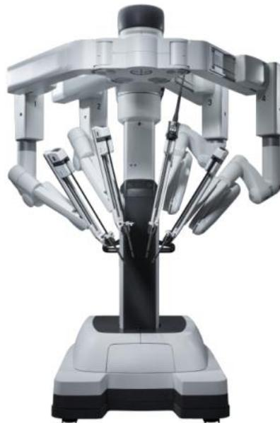
Figure 5. Da Vinci Xi surgical robot. (Source: Modern Robotics)
