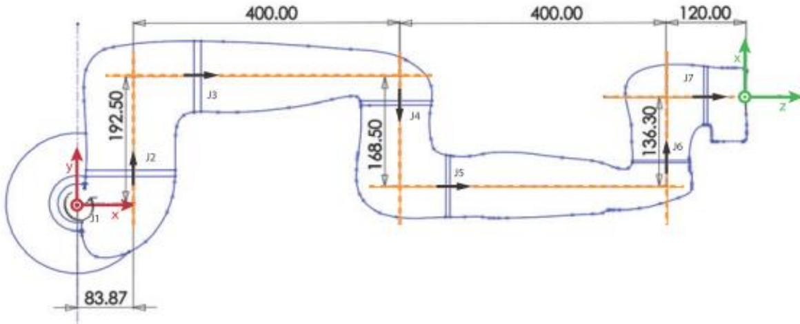
Figure 4. A top view of the Sawyer robot arm at its home configuration. Dimensions are in mm. Assume that the centerlines shown are the screw axes of the revolute joints. The  $\{s\}$  frame is at the base of the arm. The height from the base to the first joint is 317 mm. Note the joint axes are marked J1 to J7 on the diagram. (Source: Modern Robotics)
