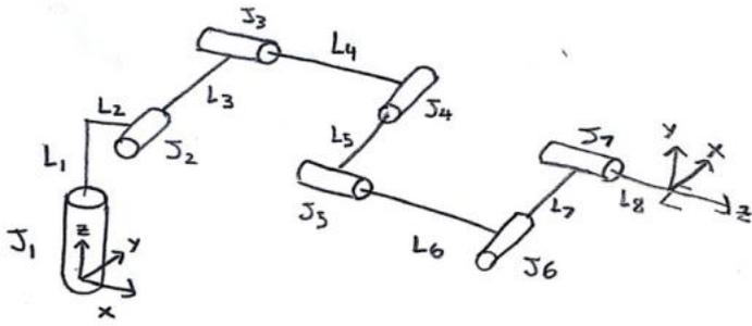
$$L_1 = 317 \text{ mm} \quad L_2 = 83.87 \text{ mm} \quad L_3 = 192.5 \text{ mm} \quad L_4 = 400 \text{ mm} \quad L_5 = 168.5 \text{ mm} \quad L_6 = 900 \text{ mm} \quad L_7 = 136.30 \text{ mm} \quad L_8 = 120 \text{ mm}$$
