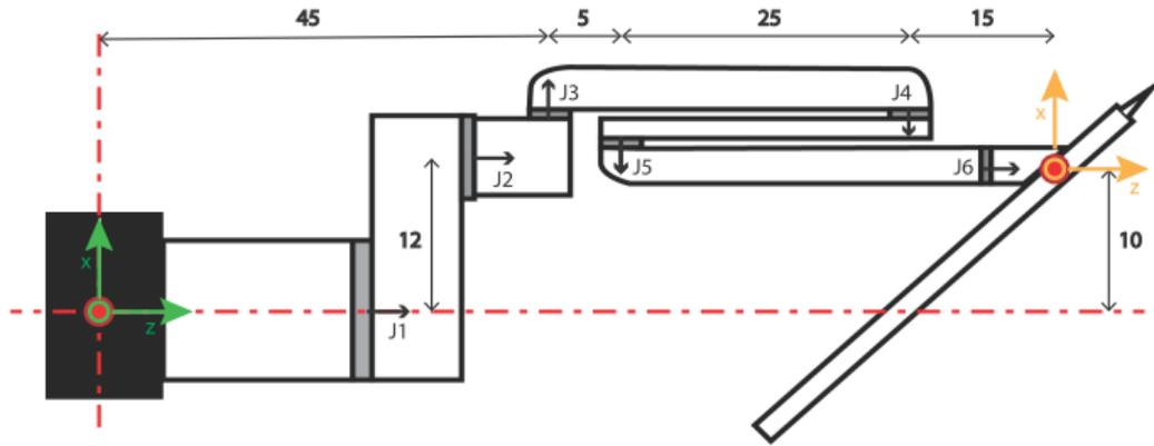
Figure 6. Top view of one da Vinci Xi surgical robot arm. Note that the grey regions represent R joints, green indicates the  $\{s\}$  frame, and yellow represents the end-effector frame  $\{b\}$  in this exercise. Dimensions are in cm. (Source: Modern Robotics)
