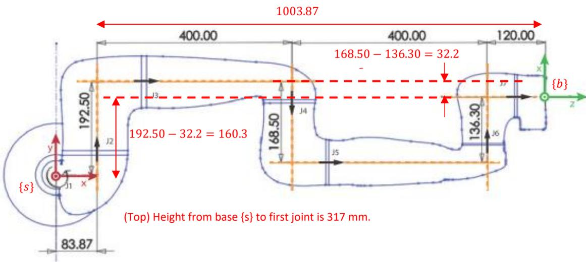
We can see that  $\{b\}$  at home configuration as shown in the figure has its  $\hat{x}_b$  along  $\hat{y}_s$ ,  $\hat{y}_b$  along  $\hat{z}_s$  and  $\hat{z}_b$  along  $\hat{x}_s$ . This gives a rotation matrix of  $R_{sb} = \begin{bmatrix} 0 & 0 & 1 \\ 1 & 0 & 0 \\ 0 & 1 & 0 \end{bmatrix}$ . The translation has three components: along  $\hat{x}_s$  is 1003.87, along  $\hat{y}_s$  is 160.3 and along  $\hat{z}_s$  is 317 giving a translation of  $t_{sb} = [1003.87, 160.3, 317]^T$ .
