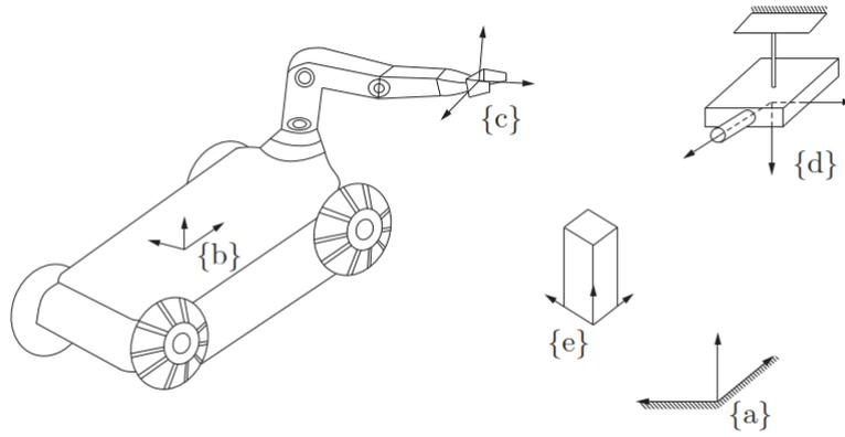
Figure 1 The fixed world frame  $\{a\}$ , the mobile robot's chassis frame  $\{b\}$ , the gripper frame  $\{c\}$ , the RGBD camera frame  $\{d\}$ , and the object frame  $\{e\}$ .
