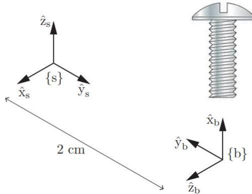
Figure 2 As the machine screw goes into a tapped hole, it advances linearly by  $4\pi$  mm every full rotation of the screw.
