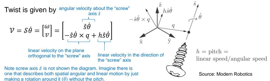
The "screw" axis  $\hat{s}$  shown in the diagram is the one in the direction of angular motion  $\omega$ , which in turn causes 2D linear motion on the plane orthogonal to the "screw" as well as a 1D linear motion in the direction of the "screw" resulting in 3D linear motion.
