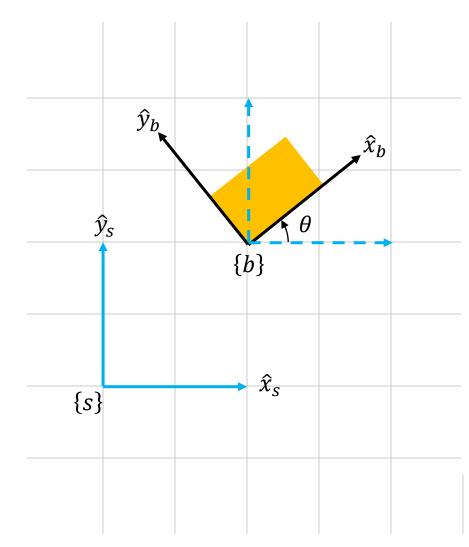
The orientation of a rigid body in space is represented by the orientation of the coordinate frame {b} attached to it, with reference to a space coordinate frame {s}.
