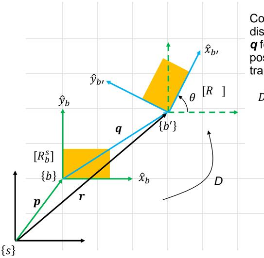
Consider a rigid body being displaced by first a translation of *q* followed by a rotation of *R*. The pose of the rigid body is transformed from frame {b} to {b'}.
