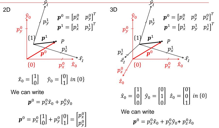
Given the same point in space, the coordinates used to represent the position of the point depend on which reference coordinate frame is being used.
