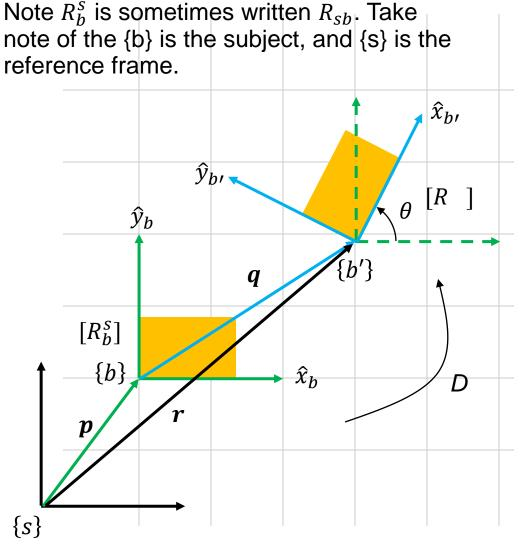
Consider a rigid body being displaced by first a translation of q followed by a rotation of R. The pose of the rigid body is transformed (displaced) from frame {b} to {b'}.
