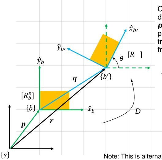
Consider a rigid body being displaced by first a translation of **p** followed by a rotation of R. The pose of the rigid body is transformed (displaced) from frame {b} to {b'}.
