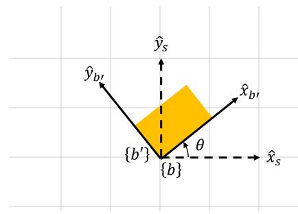
Orientation of {b'},  $R_b$ , is the result of rotating {b},  $R_b$  by the rotation expressed by R.
