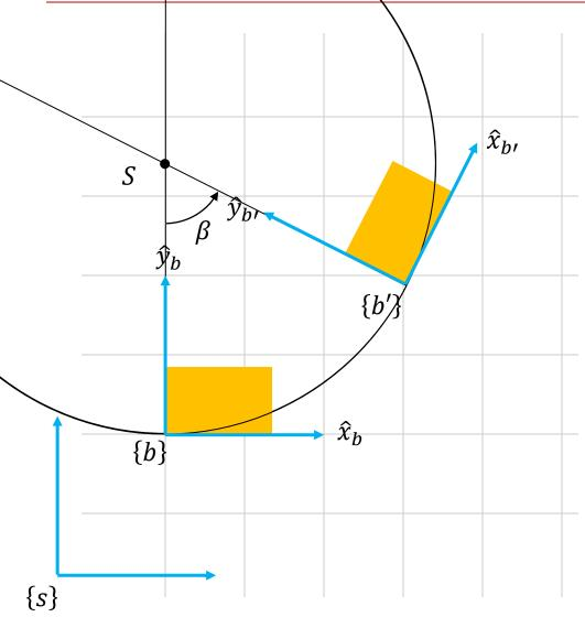
Another way of thinking of the displacement is a rotation of an angle  $\beta$  about a fixed point  $S = (s_x, s_y)$  in the space  $\{s\}$ .
