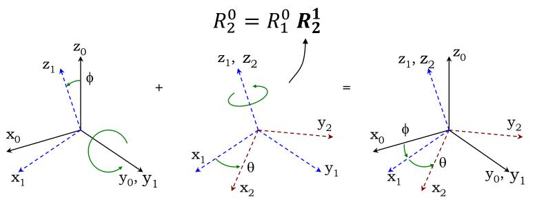
$R_j^i$  is used to denote rotation from frame **{i}** to **{j**}, which also means orientation of frame **{j}** with reference to frame **{i}**.
