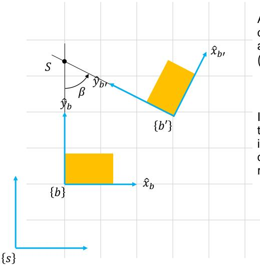
Another way of thinking of the displacement is a rotation of an angle  $\beta$  about a fixed point  $S = (s_x, s_y)$  in the space  $\{s\}$ .
