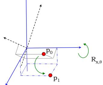
A point **p**, starting at position  $\mathbf{p}_0$  (represented as a vector) is rotated about x-axis by an angle of  $\theta$ , and its new position is  $\mathbf{p}_1$
