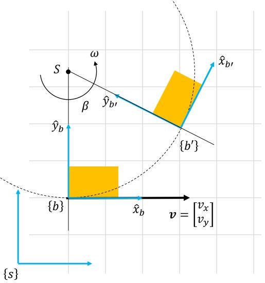
Another way of viewing screw motion is to think of it as a combination of angular  $\omega$  and linear v velocities, called **screw axis**.
