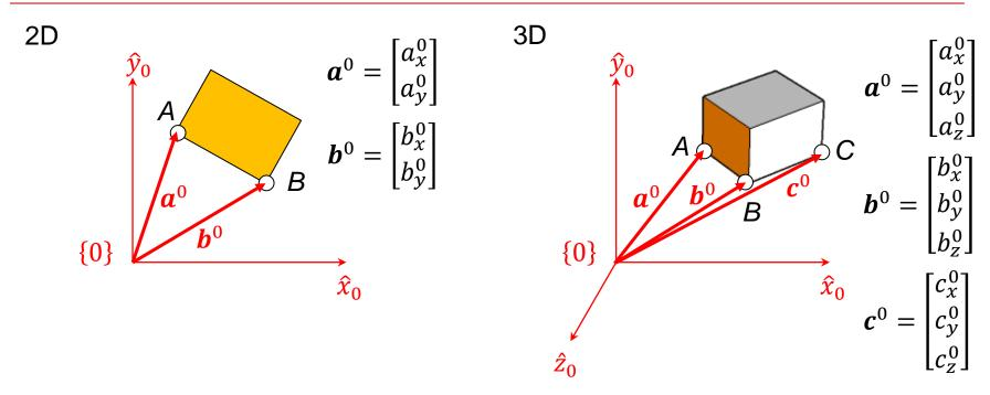
The configuration of a rigid body needs to specify where (position) it is in the space and how it is oriented (orientation).
