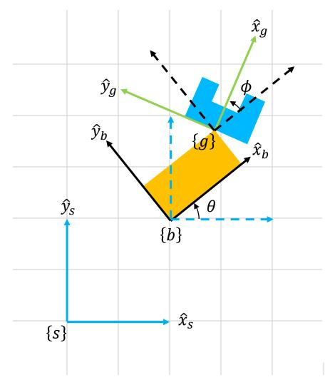
We know the orientation of the gripper represented by {g} on the effector represented {b}  $R_g^b = \begin{bmatrix} cos\phi & -sin\phi \\ sin\phi & cos\phi \end{bmatrix}$
