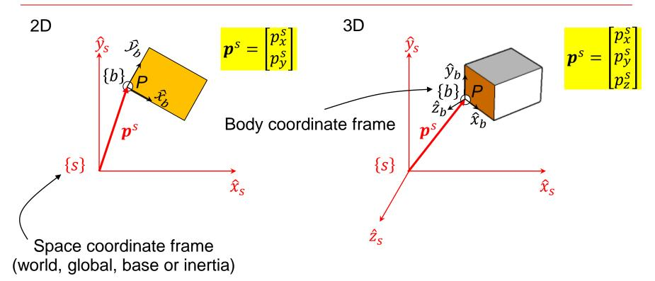
Attach a coordinate frame to the body. The origin of the body coordinate frame {b} in the space coordinate frame {s} gives the position of the body in space. The orientation of the {b} with respect to {s} gives the orientation of the body.
