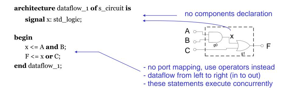
note the statements in dataflow model are based on the circuit implementation, i.e. the path of signals
