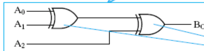
(c) 3-input odd function circuit as interconnected exclusive-OR blocks
