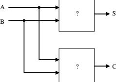
• A 1-bit Adder adds two 1-bit numbers. For two n-bit numbers, we use n 1-bit Adders.
