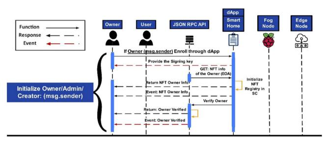
Figure 5. Sequence diagram of session connections for initializing owner representation.
